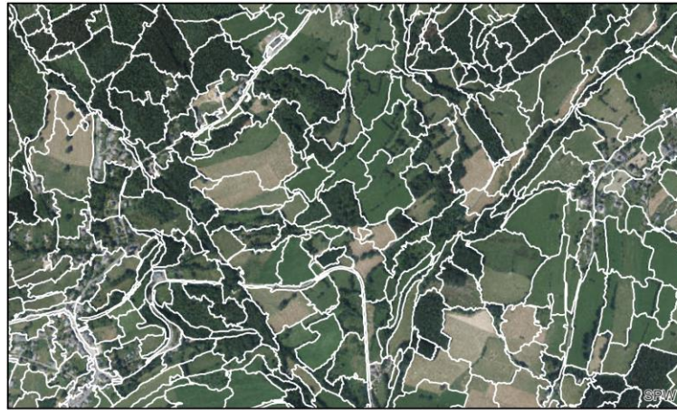
Automated image segmentation (topography and orthophotos)
